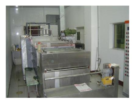
Figure 68: Film etching device at China Institute of Atomic Energy
