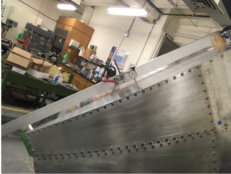
Figure 15: How the deflection of the side panel was measured.
