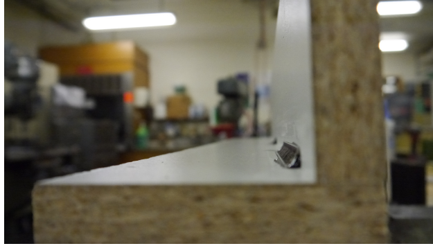
Figure 4: A bead of sealant along a test piece of wood. The bead is pushed into the seam and along the side of the wood.
