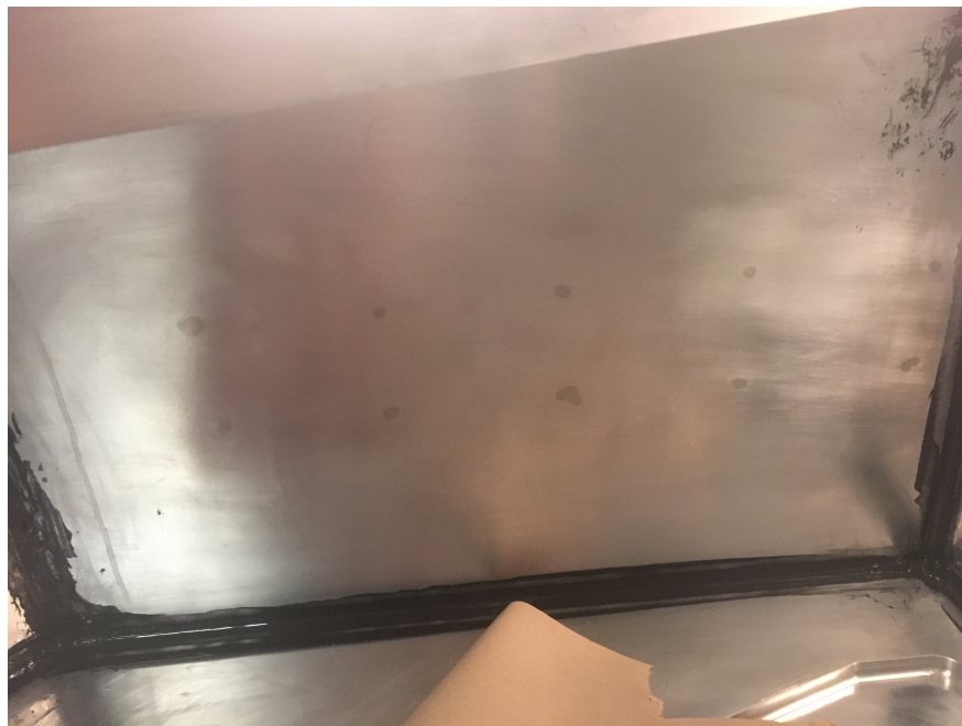
Figure 22: Discoloured blotches on the top panel.
