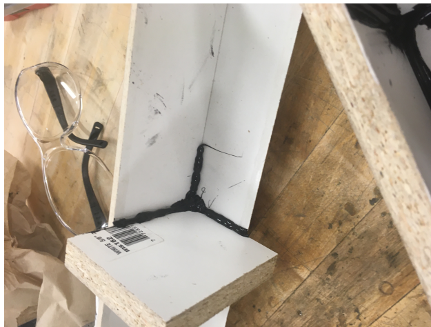
Figure 5: The bead of sealant is smaller than the first method.
