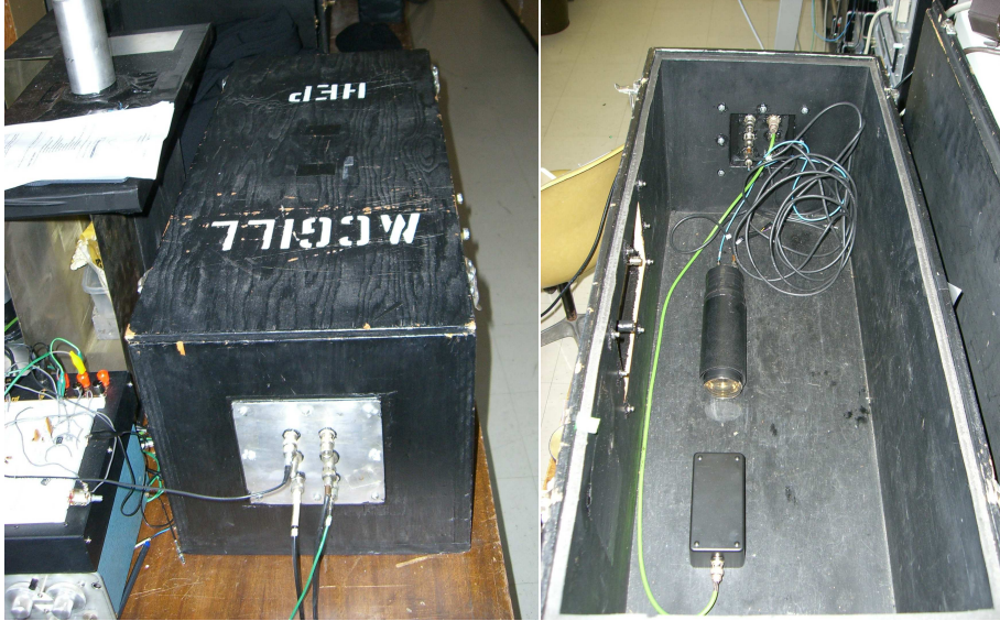
Figure 4-2: Left: The PMT and LED were located inside a light sealed box. Right: The inside of the box is shown. The green LED was located at the tip of the small black box facing the PMT and was connected in series with a 15 \pm 5 \% \Omega resistor. The PMT is encased in a \mu metal shield. During the experiment, the box was closed.
