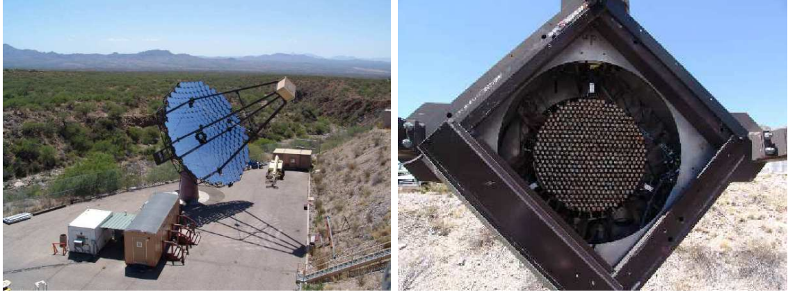
Figure 2–1: Left: VERITAS telescope 1 (of four telescopes). The buildings in the foreground are where the electronics and power supplies are located [3]. Right: Close up of VERITAS camera which is composed of 499 Photomultiplier Tubes (Model: XP2970/02) [3].
