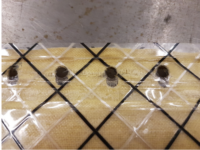
Figure 5.26: Close up of separated material layers after disassembly following Test 5.
