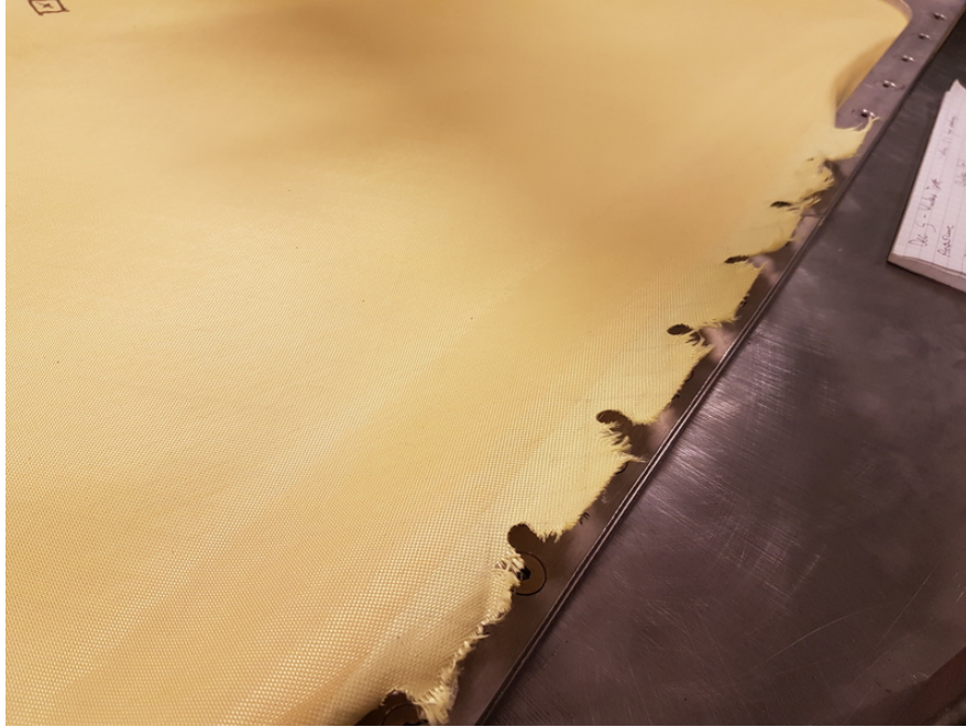
Figure 5.15: Aftermath of window failure during first Kevlar/Mylar test, focused on the portion that slipped from the flange.
