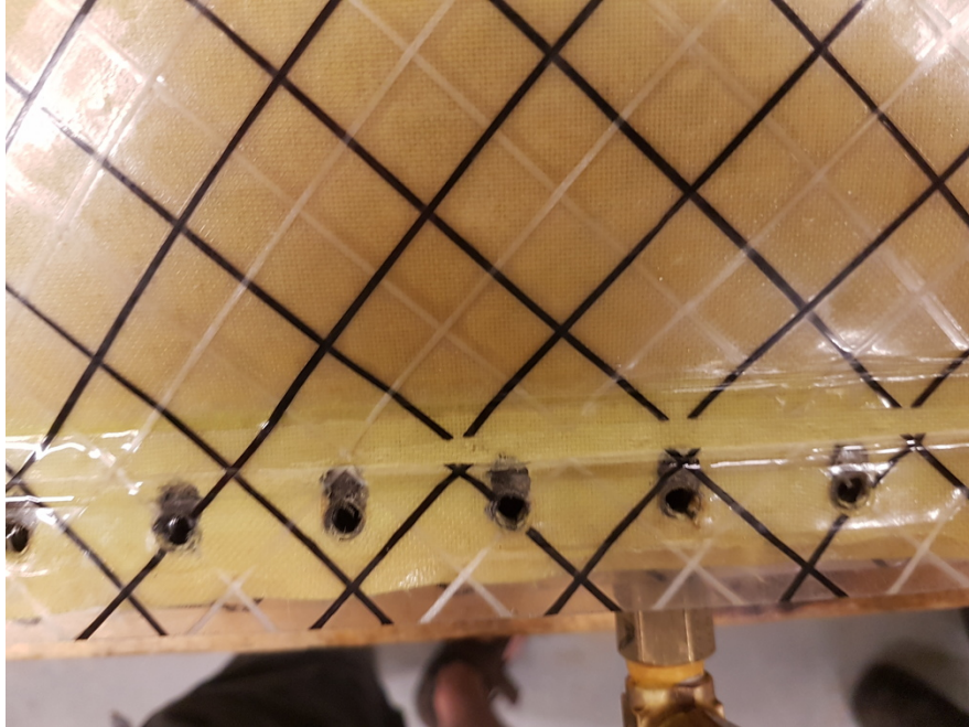
Figure 5.28: Closeup detail of damage to top Mylar layer along the location of the wire groove, after Test 6.
