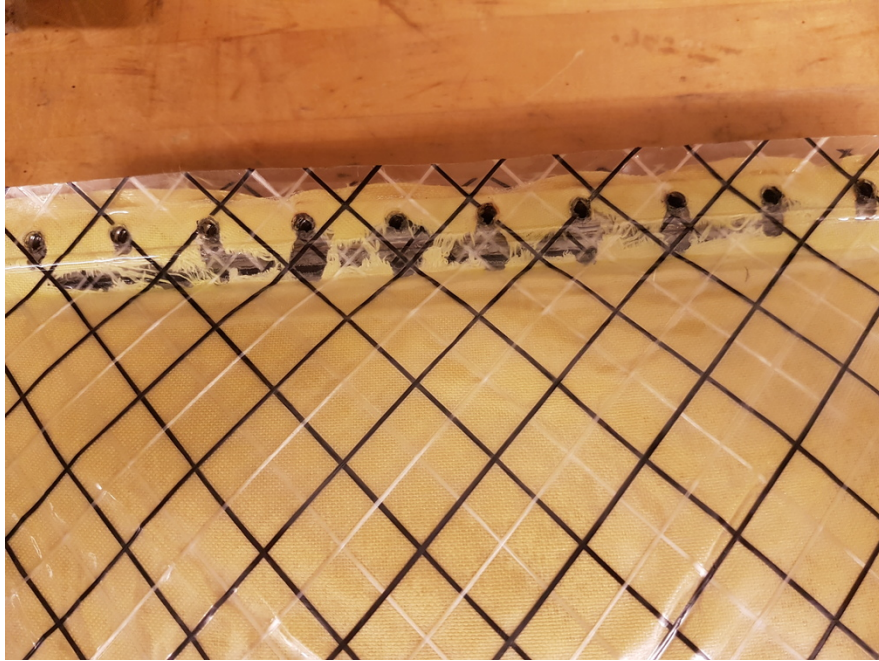
Figure 5.27: Close up of damage to Kevlar layers following Test 6.
