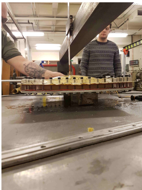
Figure 5.20: Side view of the window frame and plate, showing upward deformation at 50 psi.
