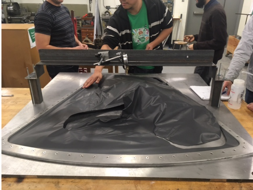
Figure 5.13: Aftermath of failure of the PET/Tedlar window.
