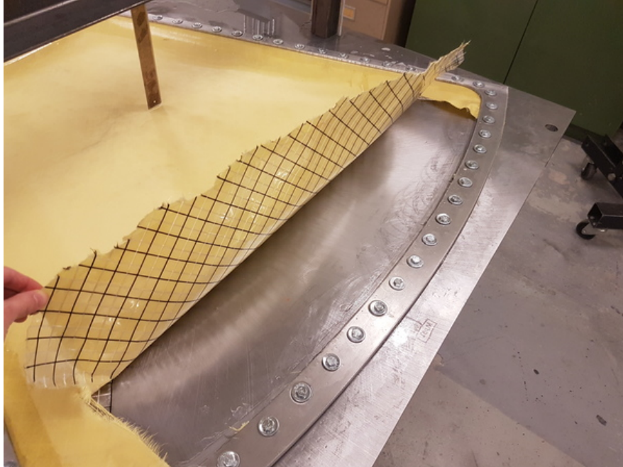
Figure 5.17: Aftermath of window failure during second Mylar/Kevlar test.
