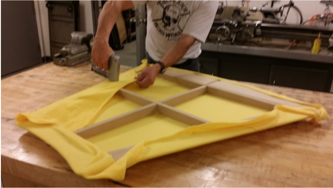
Figure 5.33: Foam cloth being stretched over the wooden frame as a mold for the full-size carbon fiber shell. The yellow color similar to the Kevlar is coincidental.
