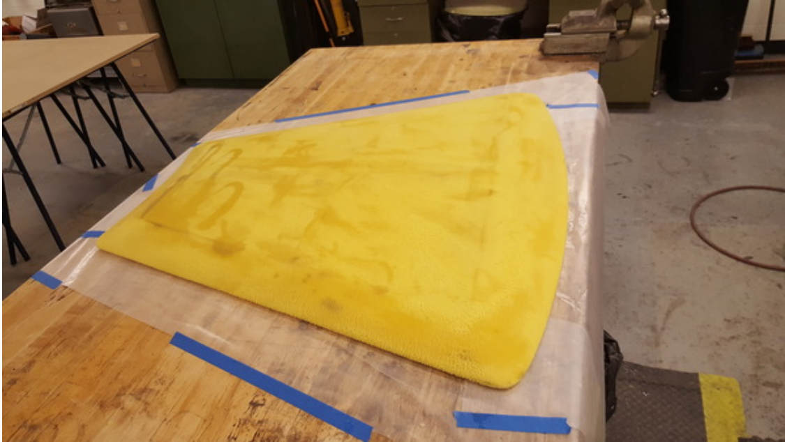
Figure 5.34: Finished mold for full-size carbon fiber shell. The yellow material is a foam cloth and similarity to the Kevlar is coincidental.
