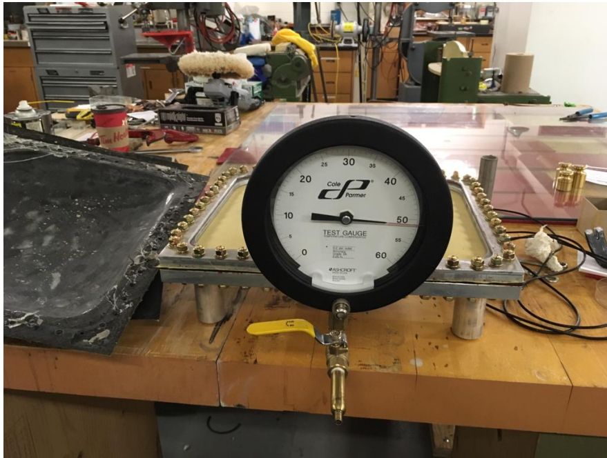
Figure 5.37: Shell 5 still under pressure after approximately one year.
