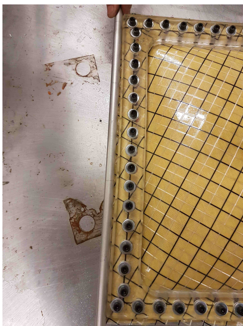
Figure 5.19: Top down view of the window frame and plate, showing inward deformation at 50 psi. A straight steel rod provides a reference.
