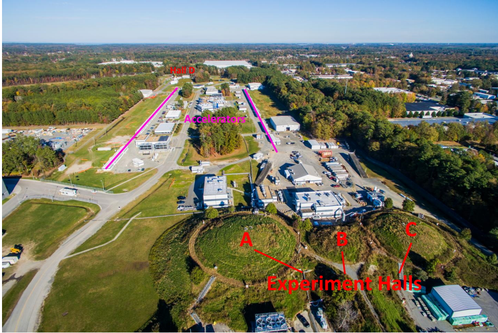
Figure 3.1: Aerial photograph of the CEBAF facility at JLab, with approximate locations of the underground experiment halls and linear accelerators marked [27].
