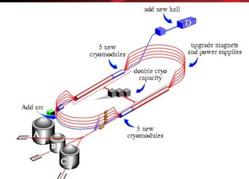
Two 1.5 GHz Superconducting Linear Accelerators provide electron beam for Nucleon & Nuclear structure studies.
