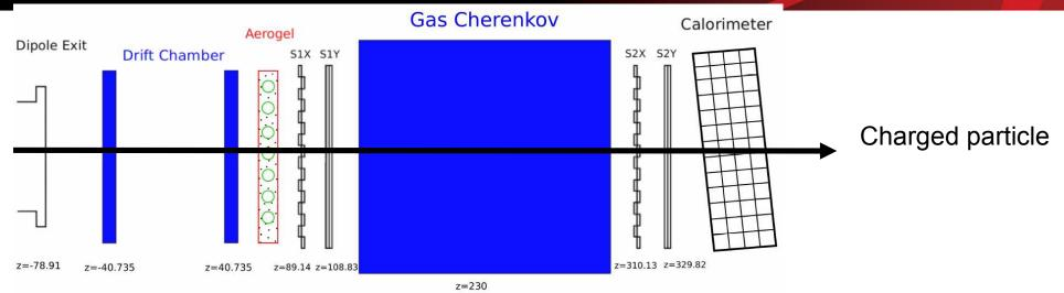
HMS focal plane detector layout, SOS is very similar Trigger: <sup>3</sup>/<sub>4</sub> planes of Hodoscopes
