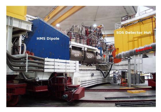
Figure 3.3: Hall C image taken during the  $F_{\pi}$ -2 experiment. The critical spectrometer and beamline components are labeled. The red "T" symbol indicates location of the target chamber. Note that the image is taken from a location between the HMS spectrometer and the beamline (downstream from the target chamber). (Original In Colour)
