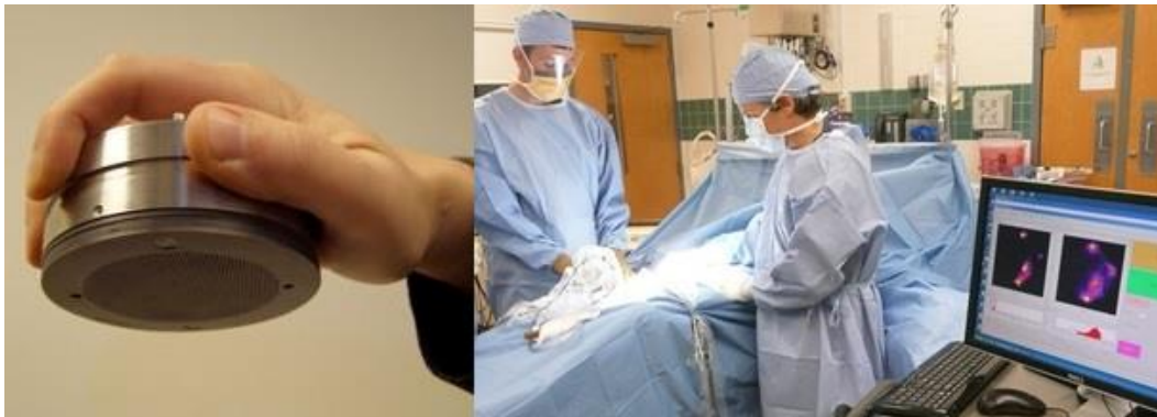
Figure 3.3.2 “Gamma Puck”: Handheld detector with a tungsten shell and tungsten collimators. A radiopharmaceutical is used to identify sentinel lymph nodes with cancer involvement during breast cancer surgery. This Jefferson Lab and University of Virginia Medical Center developed gamma camera can be used to save repeated surgeries for patients [23].
