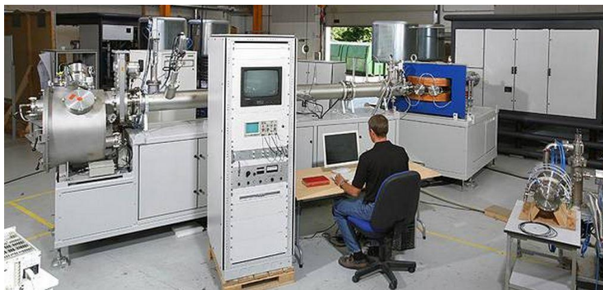
Figure 3.4.4 A 200 keV Danfysik Ion Implanter installed at the Ion Beam Materials Laboratory at LANL [60].
