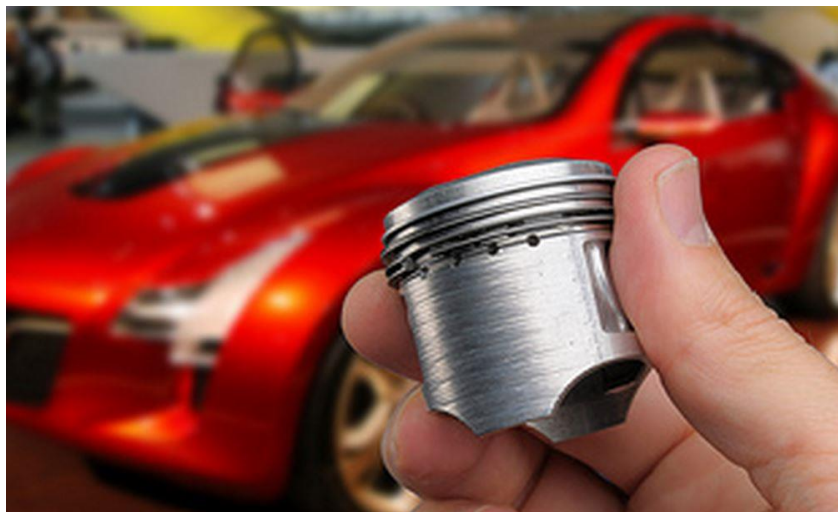
Figure 3.4.5 An automotive piston with its surface modified by electron beam bombardment to aid in oil retention [63].
