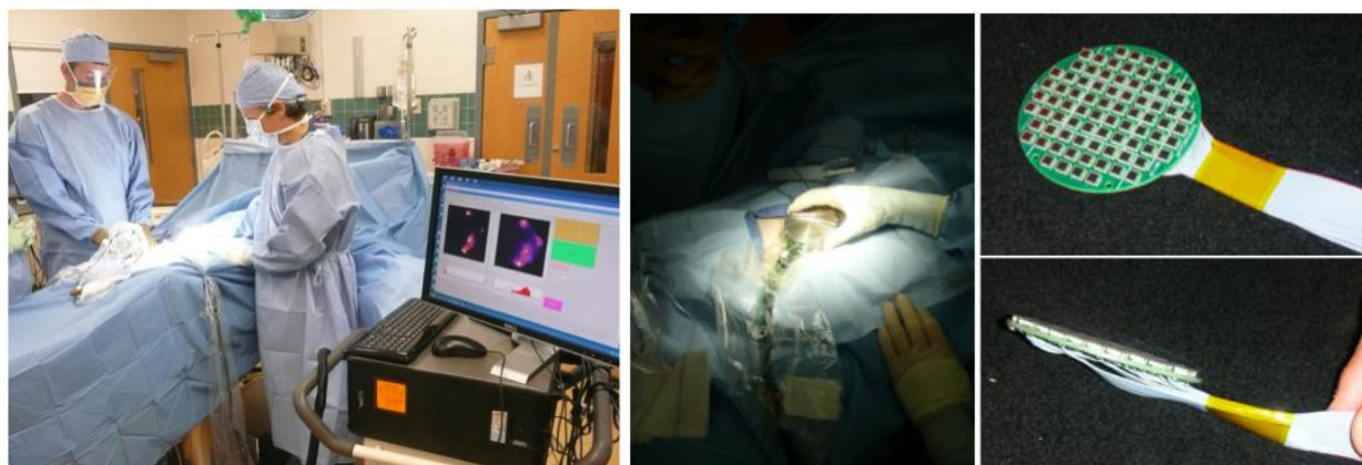
Hand-held silicon photomultiplier based gamma camera used to identify radioisotope labeled sentinel lymph nodes with cancer involvement during breast cancer surgery.
