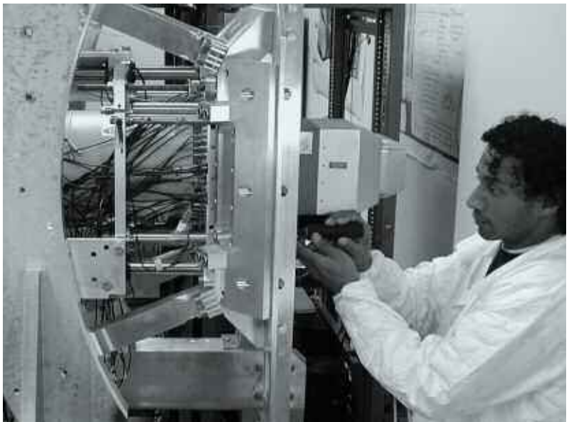
Installation of the first gamma-ray detector of the new TIGRESS spectrometer developed for the ISAC-II accelerated radioactive ion beam facility.
