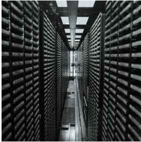
A tape robot used to access the data from Fermilab's collider experiments.
