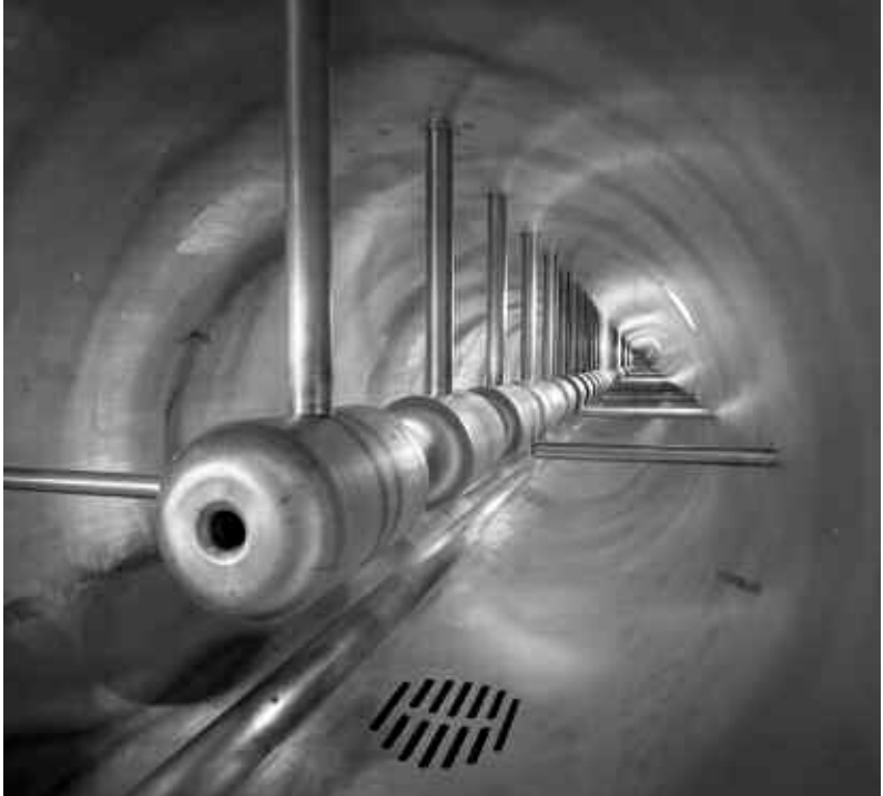
Drift tubes inside a linear accelerator at Fermilab. The beam is accelerated down the central axis of the structures.
