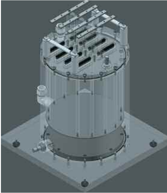
Engineering drawing of a test cell used to evaluate micropattern gas detector readout systems for Time Projection Chambers (TPCs). TPCs are likely to be used at the heart of ILC detectors and are the subject of intense R&D.
