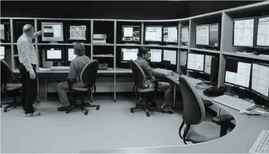
Control room of the new ISAC-II facility at TRIUMF, where beams of radioactive ions are directed to the experimental facilities.
