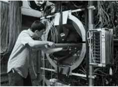
Inserting a source into the Crystal Ball detector for energy calibration. Crystal Ball is operated in Mainz, Germany by a collaboration including physicists from Mount Allison University.
