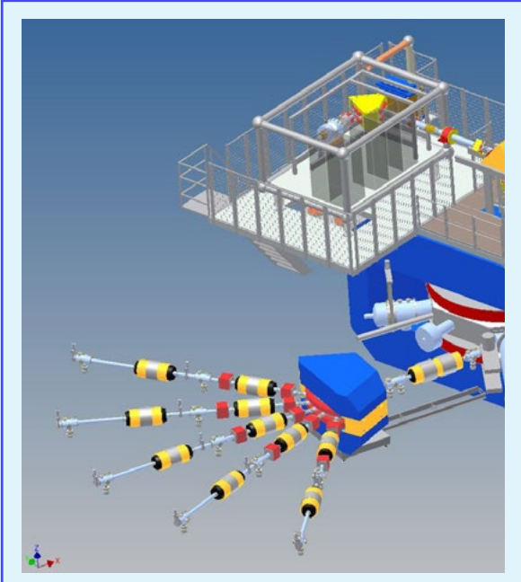
Schematic layout of the DC-280 cyclotron for the SHE Factory, Dubna, Russia
