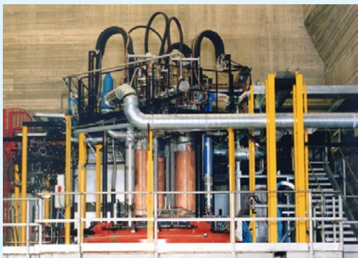
Picture of the upper part of the superconductor cyclotron at LNS, Catania, Italy
