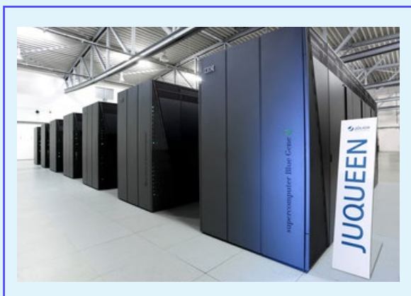
The IBM Blue Gene/Q system JUQUEEN with 5.9 Pflops peak performance at the computing center of the Forschungszentrum Jülich
