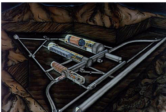
Figure 4. The Gran Sasso underground facility located off the road tunnel under the Italian Apennine mountains is home to LUNA, Europe's unique underground accelerator facility for low energy nuclear astrophysics measurements. Two accelerators have been housed at LUNA to enable nuclear reactions rates to be measured in an environment free from cosmic rays and other environmental radiation. This has enabled measurements to be extended to the low energies associated with stellar nucleosynthesis.
