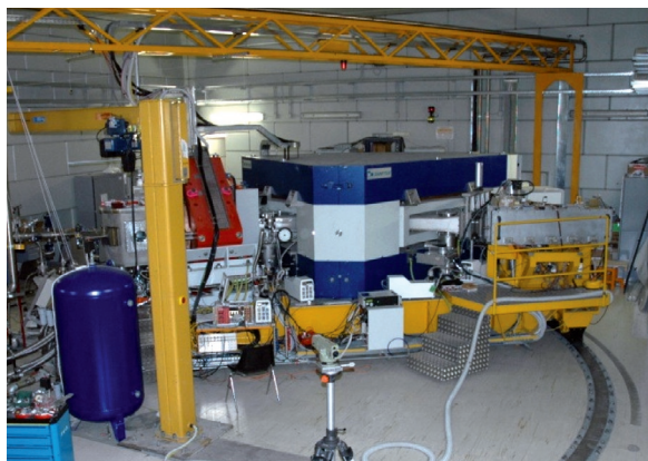
The magnetic spectrometer MAGNEX at LNS.
