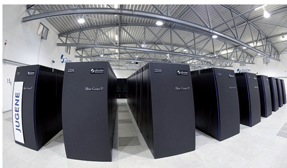
The IBM Blue Gene/P system JUGENE with 1Pflops peak performance at the Forschungs-zentrum Jülich.
