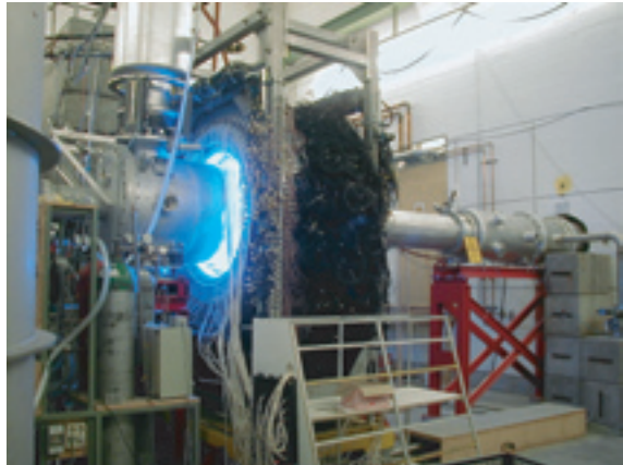
Figure 3.14: The PbF 2 -calorimeter of the A4 collaboration at the MAMI facility in Mainz.
