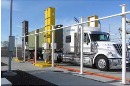
Figure 5: Portal monitor containing ^3\text{He} in use scanning a cargo containing truck
