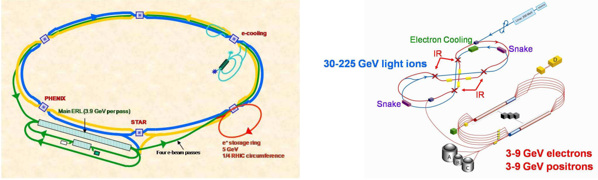
Figure 24: Design layouts of the ERL-based eRHIC, and the CEBAF-based ELIC colliders.
