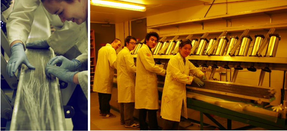
Figure 3.4: GlueX Barrel Calorimeter (BCAL) module construction by students at U. Regina.
