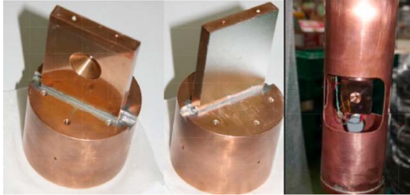
Fig. 3.1.14. Solid hydrogen target cell under development. The cell is backed by a thin silver foil.
