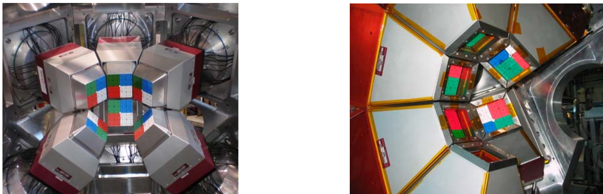
Fig. 3.1.10. Part of the TIGRESS spectrometer in the “maximum efficiency” (left) and the “optimal peak-to-background”(right) configuration.
