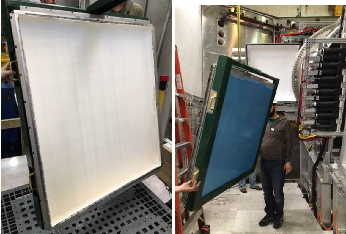
Figure 5.27: Illustration of lifting the aerogel tray to 18 degrees by hand and lifting it at into position.
