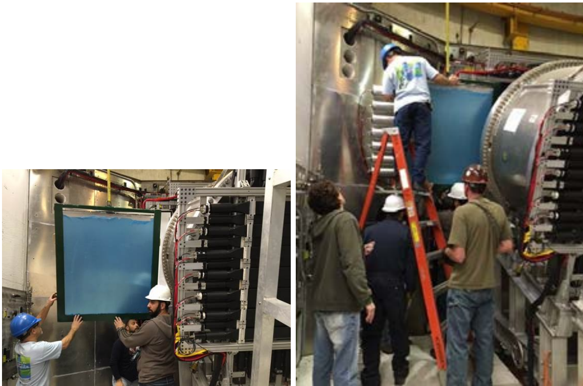
Figure 5.28: Illustration of the alignment of the aerogel tray with the diffusion box.
