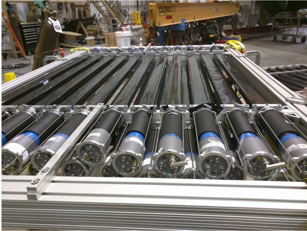
Figure 5.19: The SHMS quartz bar hodoscope plane, S2Y, before mounting into the detector stack between S2X and the pre-shower plane.
