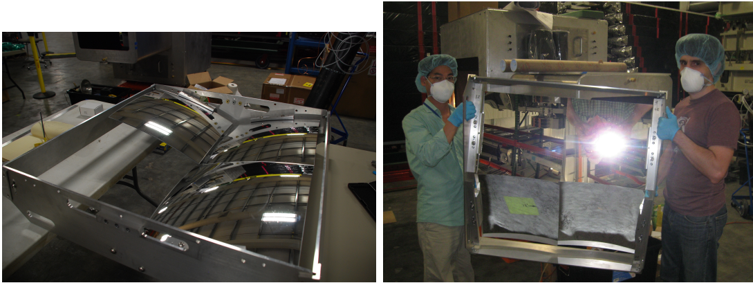
Figure 5.18: LHS: Three of four mirrors installed in frame. RHS: Frame about to be moved into tank.
