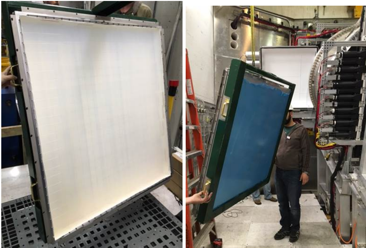
Figure 5.27: Illustration of lifting the aerogel tray to 18 degrees by hand and lifting it into position.
