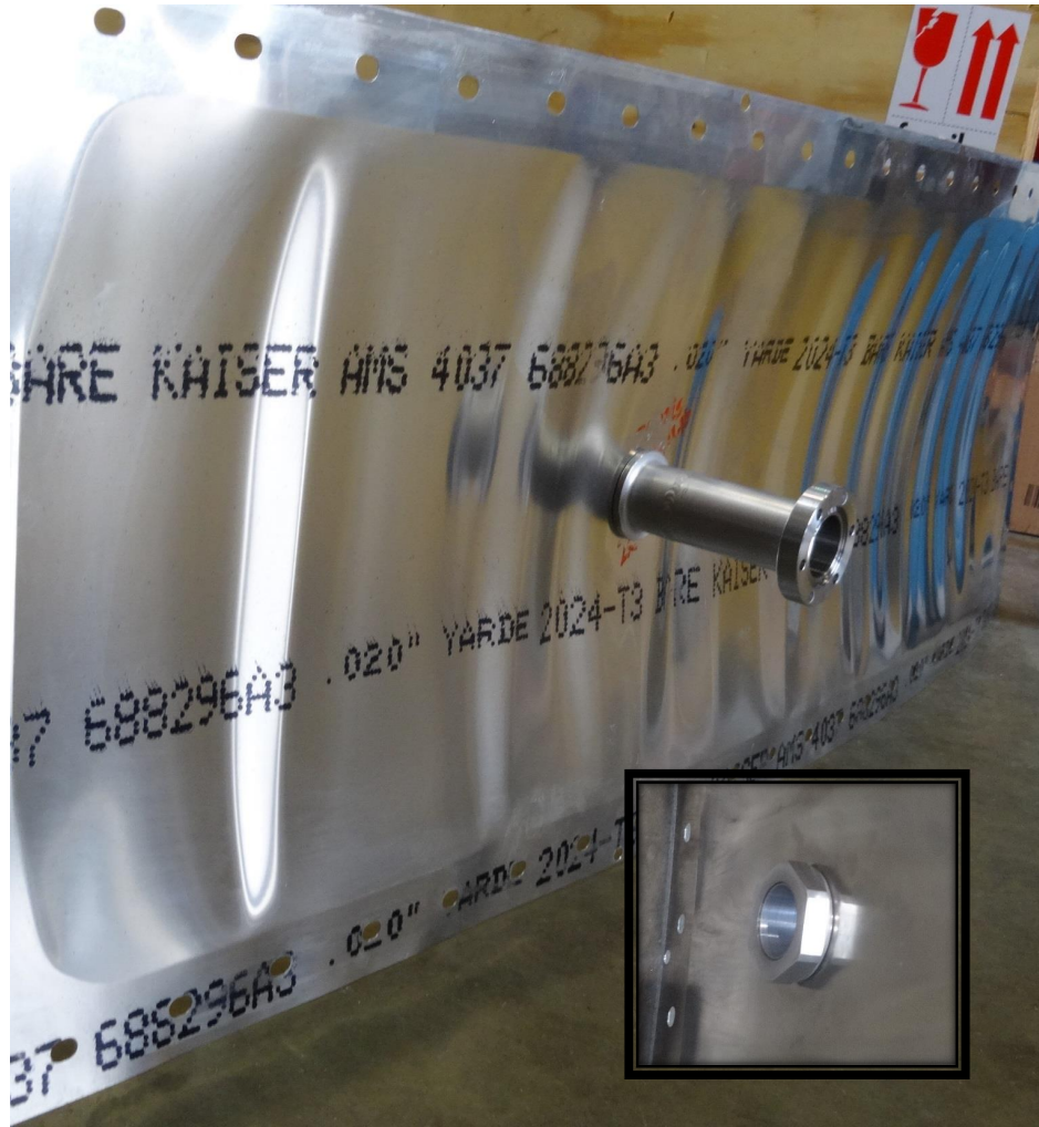
Figure 2.26: Photograph of the scattering chamber window with the short exit beam pipe attached. The inset shows the nut on the opposite side (the vacuum side) attaching this beam pipe to the window.
