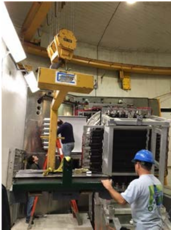
Figure 5.26: Aerogel tray on the pallet picked up by the crane.
