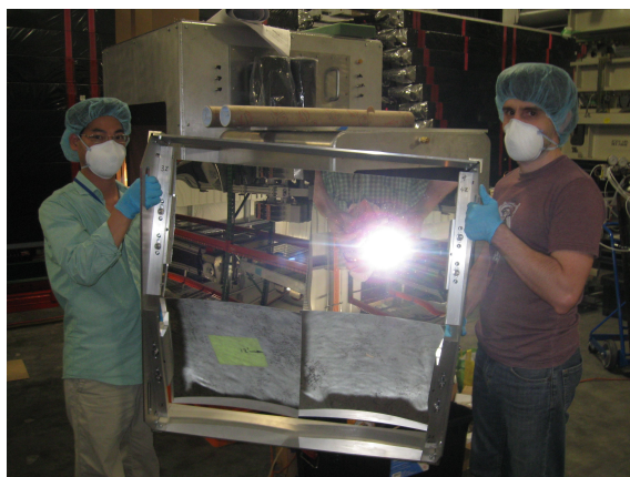
Figure 37: Frame with mirrors about to be moved into tank.
