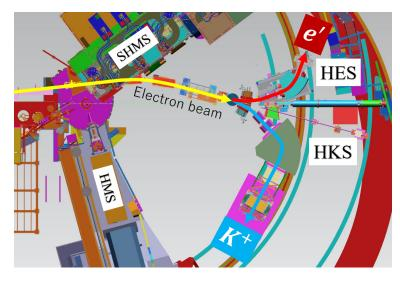
FIG. 16. Schematic of one concept for the experimental setup for hypernuclear missing-mass spectroscopy Hall C. A scattered electron and  $K^+$  from the  $(e, e'K^+)$  reaction are measured in HES and HKS, respectively. HES is bending horizontally in the figure, however the vertical bending option is being considered for extended gas targets.
