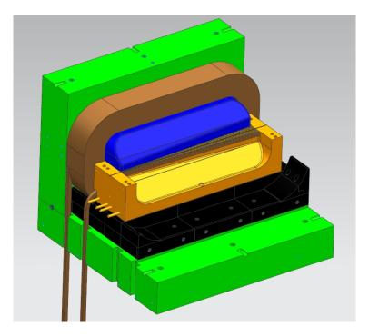
FIG. 7. A CAD rendition of the Compact Photon Source (CPS) without its external shielding and part of yoke removed for clarity. From inside to outside: the slotted Cu power absorber is shown in yellow; the magnet pole is blue; the WCu inner shielding is black, the magnet coil is brown, and the magnet yoke is green.
