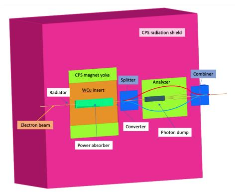
FIG. 17. The layout of the positron/electron beam source with CPS.
