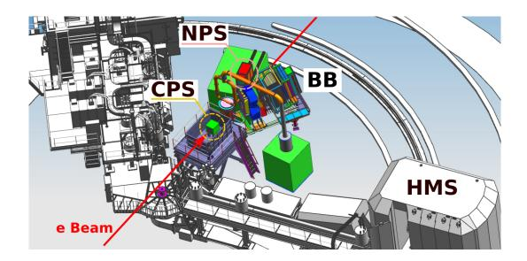
FIG. 2. Here the base equipment focusing spectrometers are temporarily parked at large angles, making room for a proton Compton scattering experiment. Downstream of the standard pivot in this example are located the Compact Photon Source (CPS), a polarized proton target, and the large acceptance spectrometers Bigbite (BB) and the Neutral Particle Spectrometer (NPS).
