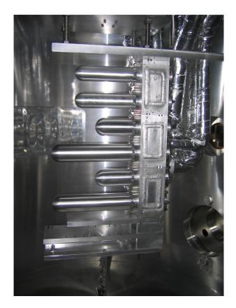
FIG. 3. The cryotarget configuration. Each independent loop has 2 cell lengths available. Cell lengths of 4cm, 10cm, and 15cm appear in this photo. The solid target ladder is suspended from the bottom.
