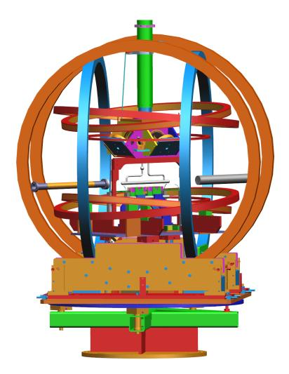
FIG. 4. CAD rendering of a polarized <sup>3</sup>He target configuration used in Hall C. The <sup>3</sup>He target cell is the horizontal grey cylinder in the center of the frame. The large rings oriented vertically and horizontally make up three independent pairs of Helmholtz coils which provide polarizing magnetic fields in arbitrary direction. Laser power for optical pumping of the target is directed from the top of the frame to the pumping chamber above the target cell.
