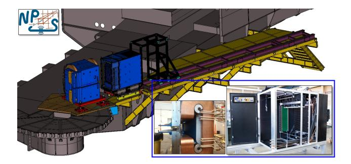
FIG. 8. A CAD rendition of the Neutral Particle Spectrometer (NPS). Scattered particles enter from the left. A sweeping magnet is located in front of the calorimeter to help suppress background from low energy electrons. Inset photos: (left) a close-up of the sweeping magnet, and (right) the cabinet which provides temperature stabilization and access to the phototubes and the many HV, signal, and fiber optic cables.
