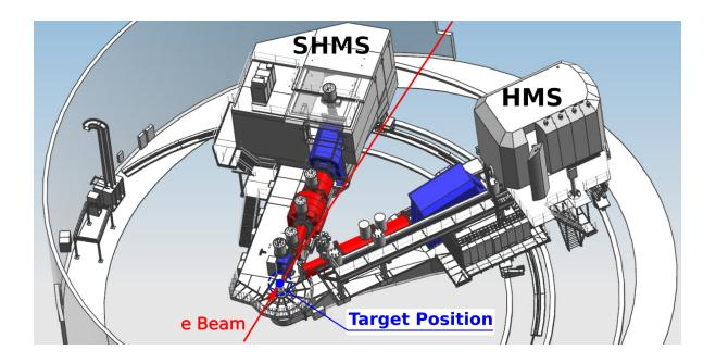
FIG. 1. Hall C overview. The beam enters diagonally from lower left. In this example, the base equipment focusing spectrometers HMS and SHMS are configured for a coincidence (e,e' hadron) experiment.
