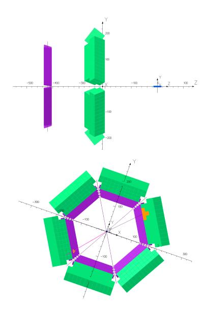
FIG. 20. Top panel: Side view of the apparatus. The electron beam goes from right to left. The proton detector is shown in green and the electron detector in purple; the liquid hydrogen target is shown in blue. Bottom panel: Front view of the apparatus. The blocks in orange get signals from the electron and the proton whose directions are shown in red.
