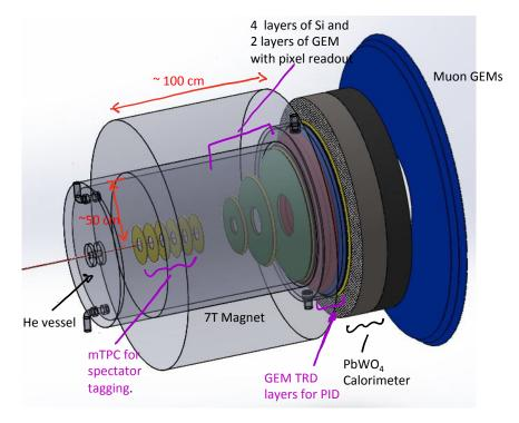
FIG. 13. A CAD rendition of the proposed compact solenoid spectrometer. The bore of the magnet will be filled with helium gas at STP to reduce multiple scattering. The target will be located at the center of the mTPC. The calorimeter and the muon chambers could be moved further downstream to reduce pile-up in the calorimeter as needed.
