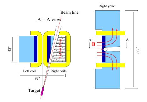
FIG. 10. The concept of the SBS magnet [40]. The left figure is a top view of a horizontal crosssection through the magnet center. The right figure is a side view of the right yoke looking downstream which shows the slot which has been machined to allow the SBS to reach small angles with respect to the primary electron beamline.
