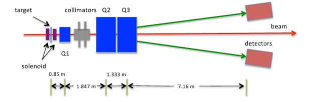
FIG. 5. Layout of the Hall C Møller polarimeter. A pure iron foil is polarized out-of-plane in a high field, split-coil solenoid magnet while a quadrupole-based magneto-optical system (Q1, Q2, Q3) focuses the scattered and recoiling electrons on a pair of lead glass calorimeters about 11 m downstream.
