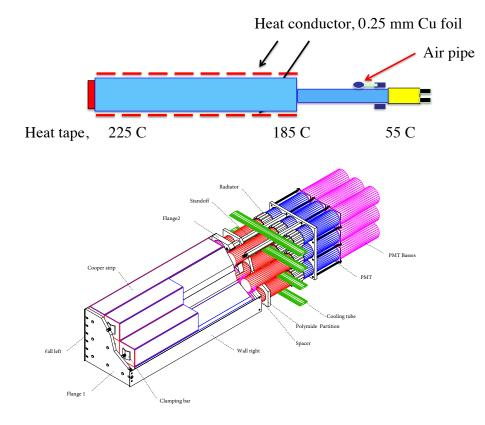
FIG. 12. Top - An individual heated block in ECAL. Bottom - A module of  $3 \times 3$  blocks.
