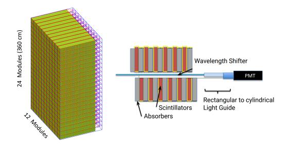
FIG. 11. (Left panel) Schematic of the 288-block assembly, and (right panel) the method of light collection in an individual HCAL module.
