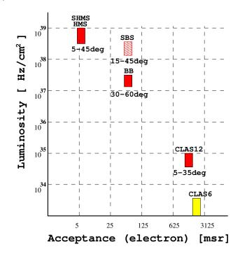
FIG. 9. The maximum luminosity vs acceptance landscape for magnetic spectrometers at JLab [30].
