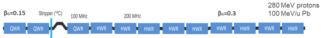
Figure 5.9: Schematic layout of the SRF section including a stripper section after the second QWR module.
