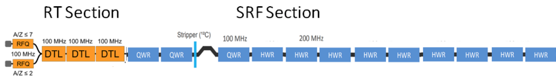
Figure 5.2: Overall layout of the JLEIC injector linac.
