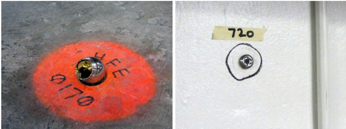
Figure 10.4: Floor Monument and 1.5 inch sphere (left). Wall Monument (right).
