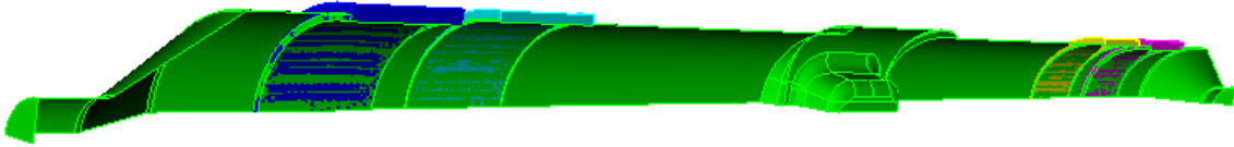
Figure 6.211: The 394 MHz WOW RFD crab cavity with beam line absorbers, 2 on each side of the cavity.
