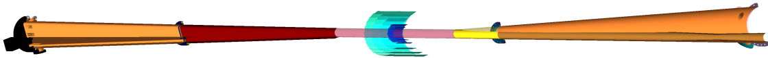
Figure 8.8: GEANT4 model of IR1 Beam Pipe, with Si Vertex Tracker. The electron beam enters horizontally from the right, and exits in the rectangular beam channel to the left. The ion beam enters in the small tube on the lower left, and exits via the large cone on the upper right.
