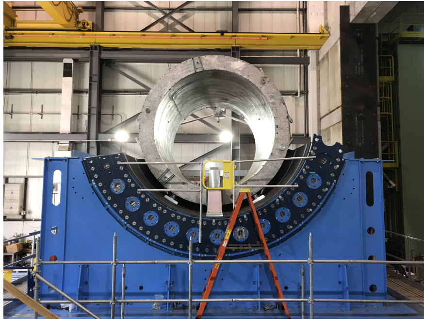
Figure 2.3: The BaBar solenoid in October 2021, during installation in the sPHENIX experiment. The solenoid is resting in the barrel outer hadronic calorimeter and flux return, which will be completed with additional sectors in the coming months. The barrel flux return (outer hadronic calorimeter) and BaBar solenoid are items planned to be reused by the ECCE experiment. The experimental cradle may also be reused.
