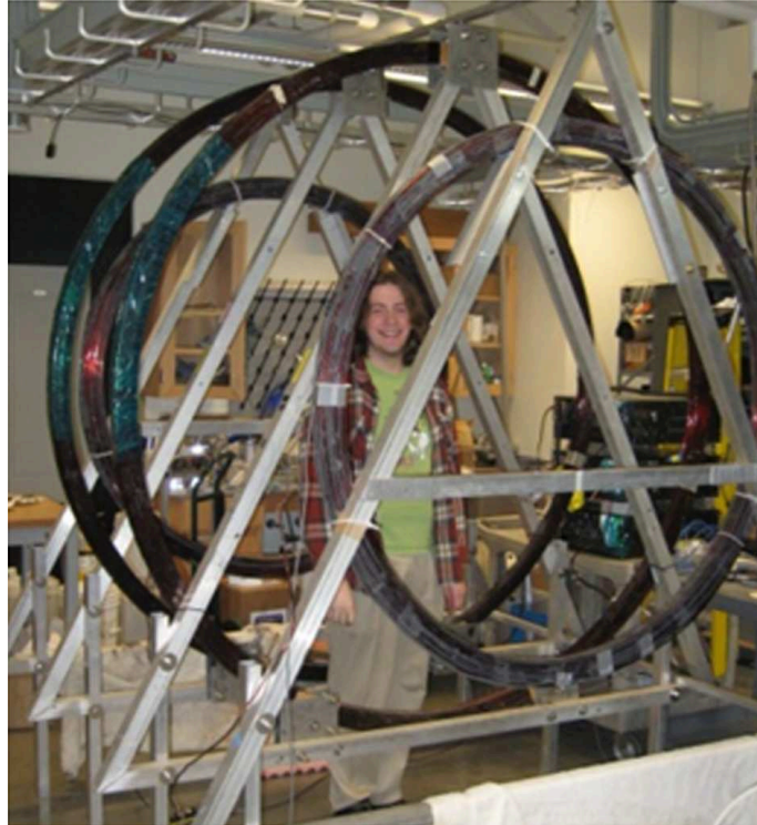
FIG. 18: Large 1.8 m magnetic field coils achieve 75 Gauss with 10^{-3} uniformity.
