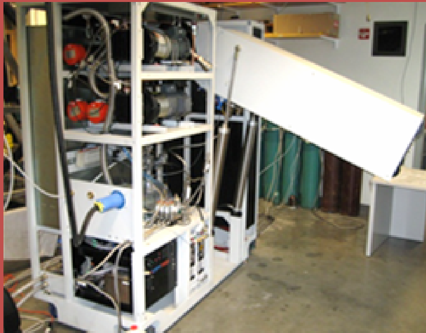
Assembled, Operating ^3\text{He} Polarizer
