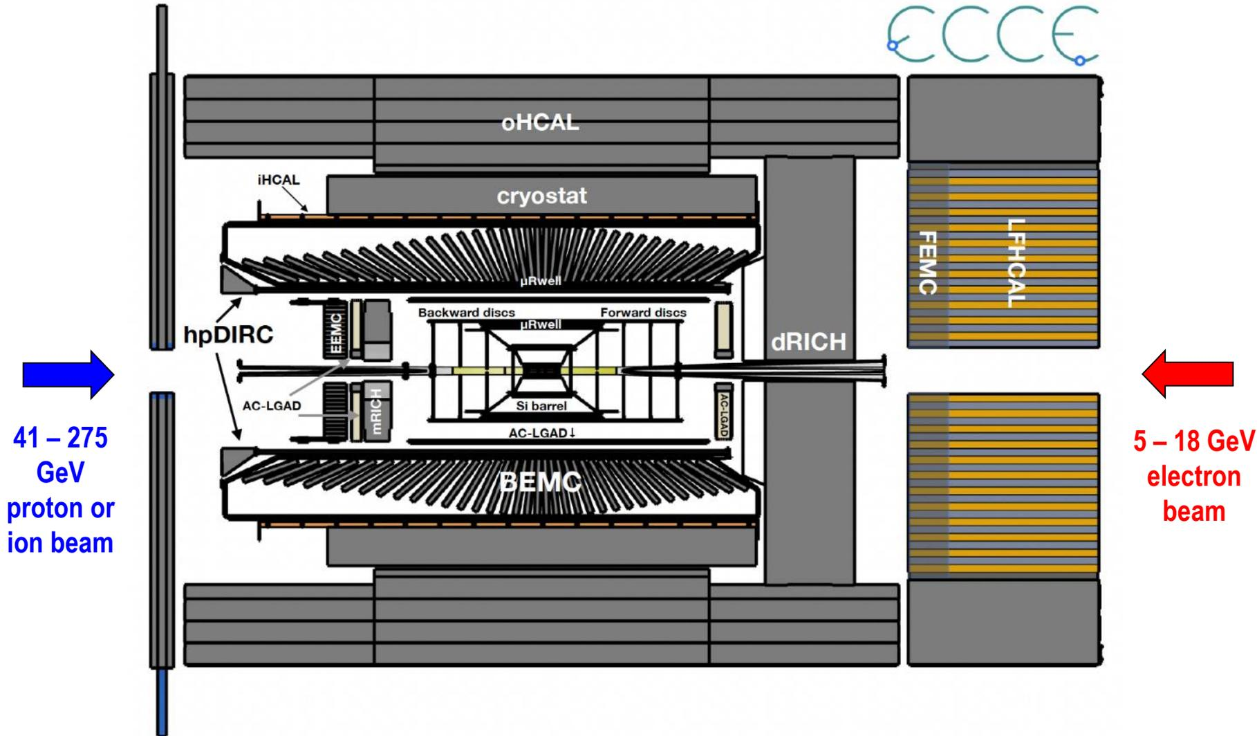
Solenoid: superconducting 1.5T 3.5m(length) x 1.5m(radius) from SLAC BaBar
