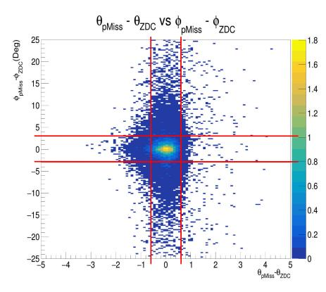
Differences between hit and calculated neutron positions on ZDC for DEMP events
