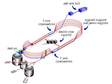
Two 1.5 GHz Superconducting Linear Accelerators provide electron beam for Nucleon & Nuclear structure studies.
