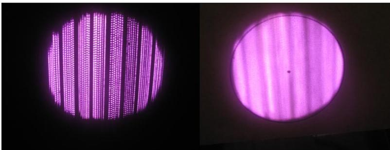
48 Bar exit beam, and 1m downstream with diffuser. Divergence ~3x6 mrad (hor x vert.)
