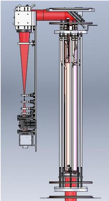
K:Rb Hybrid Spin Exchange Optical Pumping
