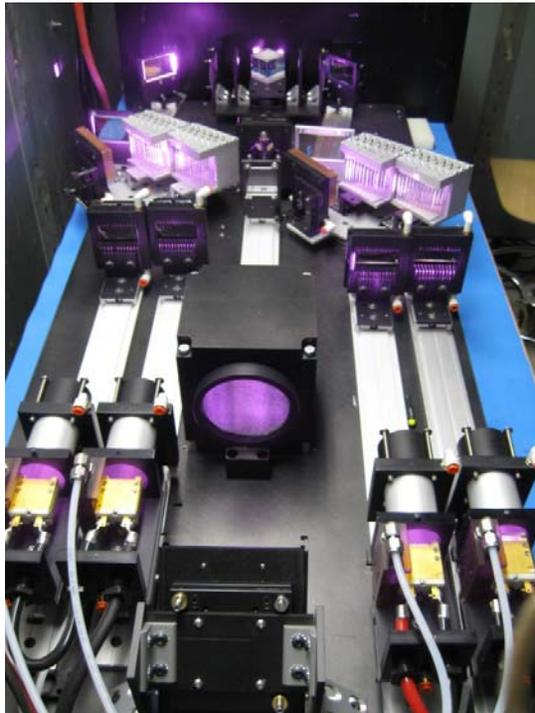
Four 12 bar lasers (foreground) combining their outputs into a single 10 cm diameter beam (center).
