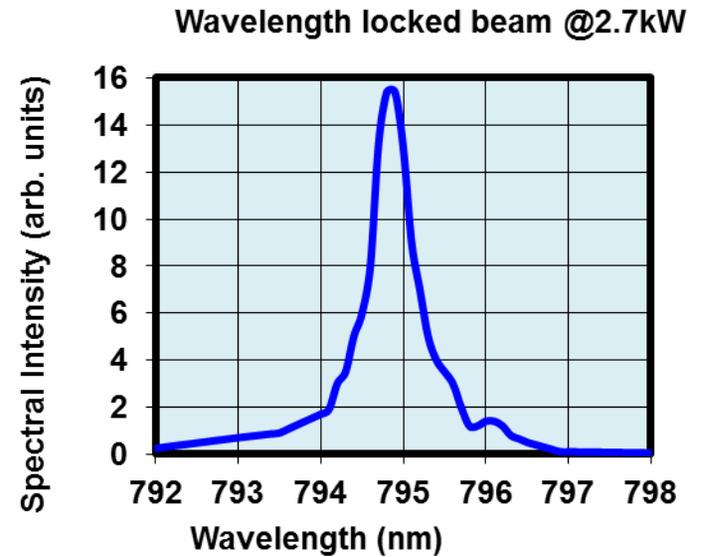
Power 0.6 nm narrowed laser (max = 110A)
