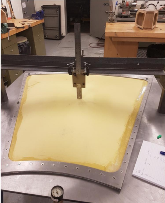
Photo of 2nd test setup with epoxy around circumference, which gave better performance.
